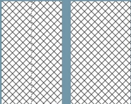
The image shows two diamond-shaped grid patterns. The left one is labeled 'Standard scanner' and the right one is labeled 'ROWE Scan 450i'. The ROWE pattern appears more uniform and consistent in spacing.
